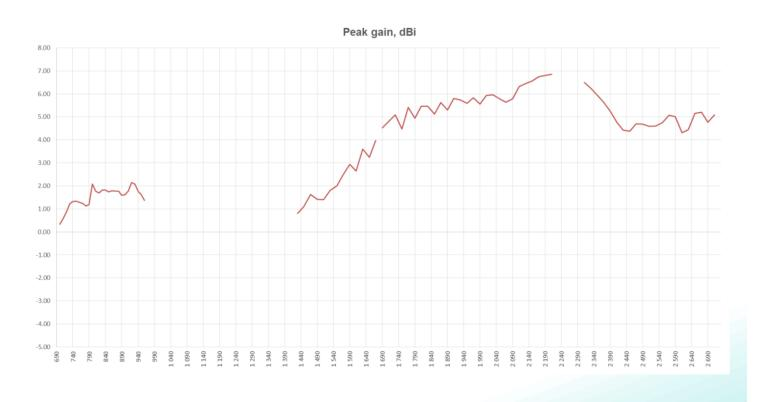
From datasheet for Pulse W3796 antenna
