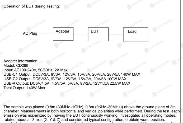
rotated about all 3 axis (X, Y & Z) and considered typical configuration to obtain worst position, manipulating interconnecting cables, rotating the turntable, varying antenna height from 1m to 4m in both horizontal and vertical polarizations. The emissions worst-case are shown in Test Results of the following pages. The worst case is X position.
