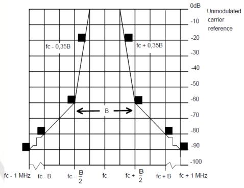
fc = Transmitter carrier frequency
