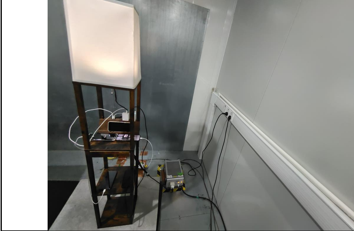
Conducted Emission Test Setup
