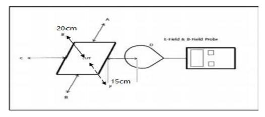
Note: Measurements should be made from all sides and the top of the primary/client pair, with the 20 cm measured from the center of the probe(s) to the edge of the device.
