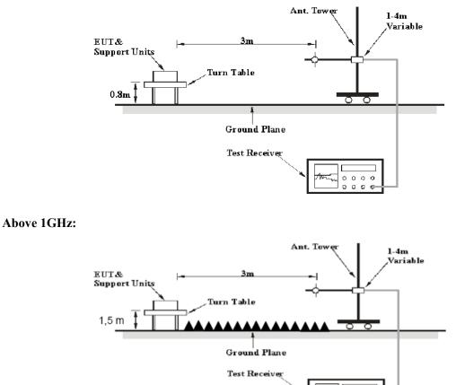
The radiated emissions were performed in the 3 meters distance, using the setup accordance with the ANSI C63.10-2013. The specification used was the FCC 15.209, and FCC 15.247,RSS-247,RSS-Gen limits.
