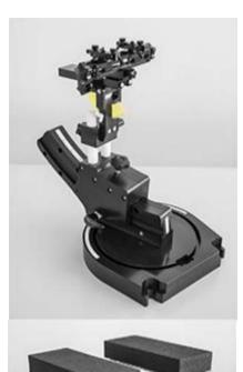
The DASY device holder is designed to cope with the different positions given in the standard. It has two scales for device rotation (with respect to the body axis) and device inclination (with respect to the line between the ear reference points). The rotation center for both scales is the ear reference point (ERP). Thus the device needs no repositioning when changing the angles.
