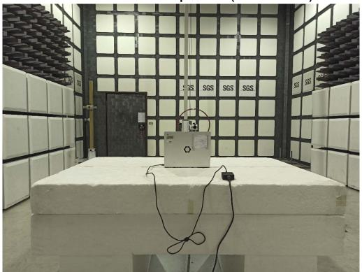
Radiated Emission Set up Photos (Below 1GHz)
