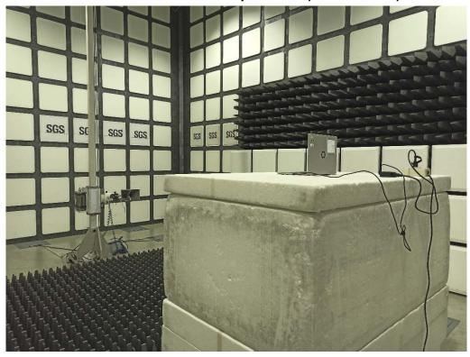
Radiated Emission Set up Photos (Front View)
