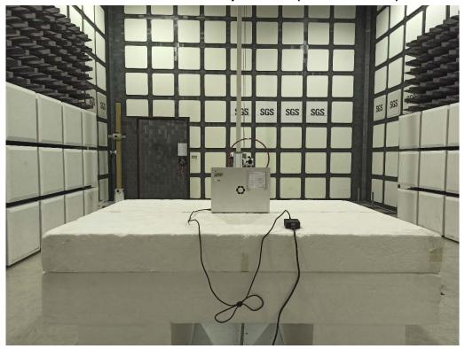
Radiated Emission Set up Photos (Below 1GHz)
