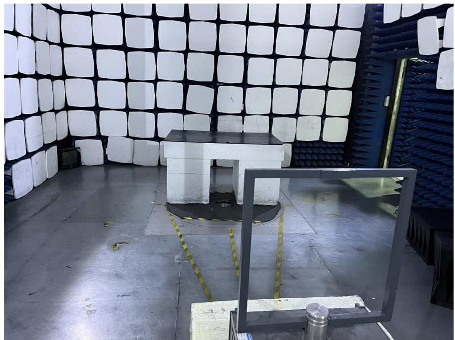
Radiation Emission Test Setup (Below 30MHz)
