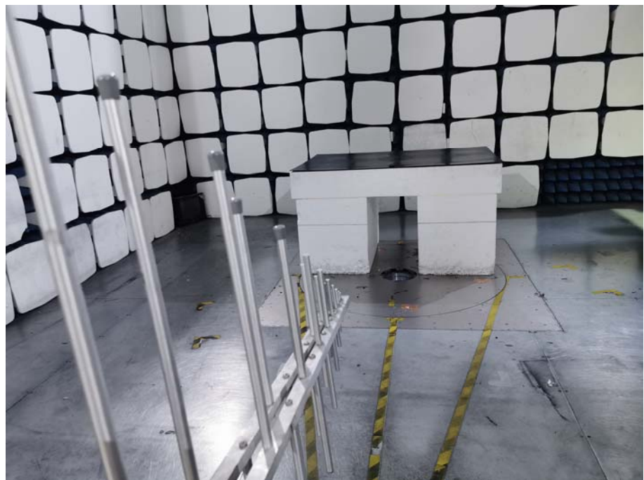
Radiation Emission Test Setup (30MHz to 1GHz)
