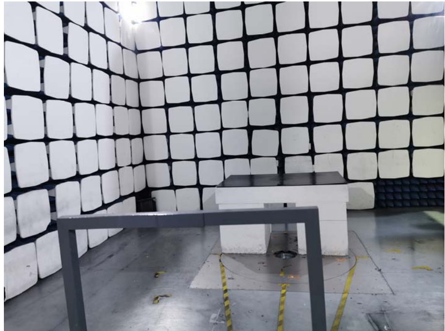
Radiation Emission Test Setup (Below 30MHz)
