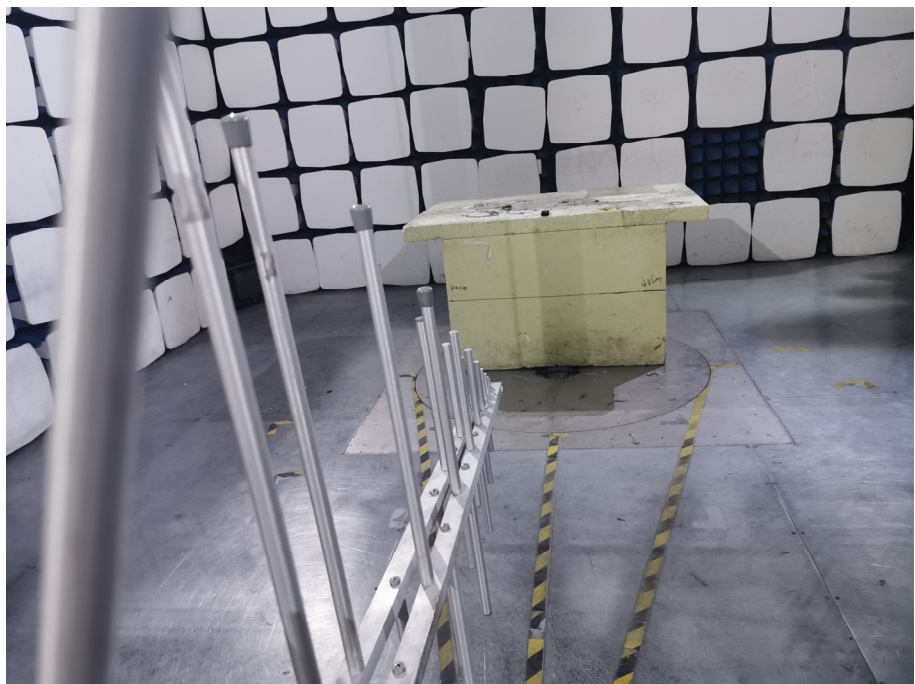
Radiation Emission Test Setup (30MHz to 1GHz)
