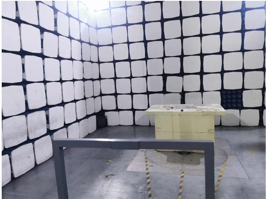
Radiation Emission Test Setup (Below 30MHz)
