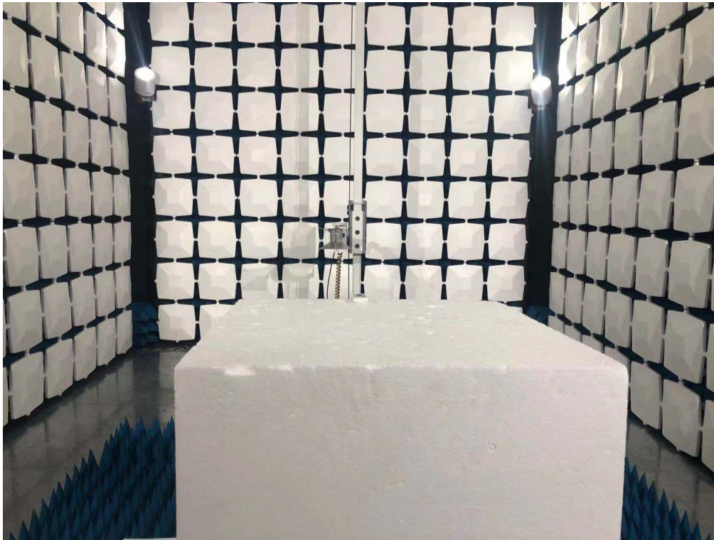
Above 1GHz for radiated emission test setup
