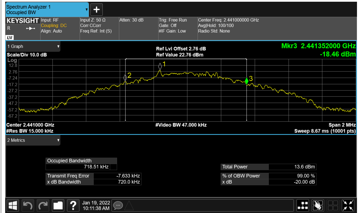
-20dB Bandwidth NVNT 1-DH1 2480MHz Ant1
