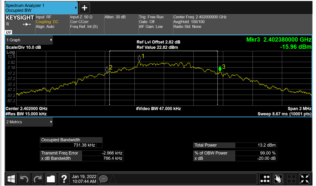
-20dB Bandwidth NVNT 1-DH1 2441MHz Ant1
