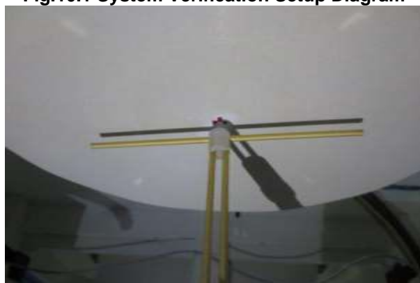
Fig.10.2 Photo of Dipole setup
