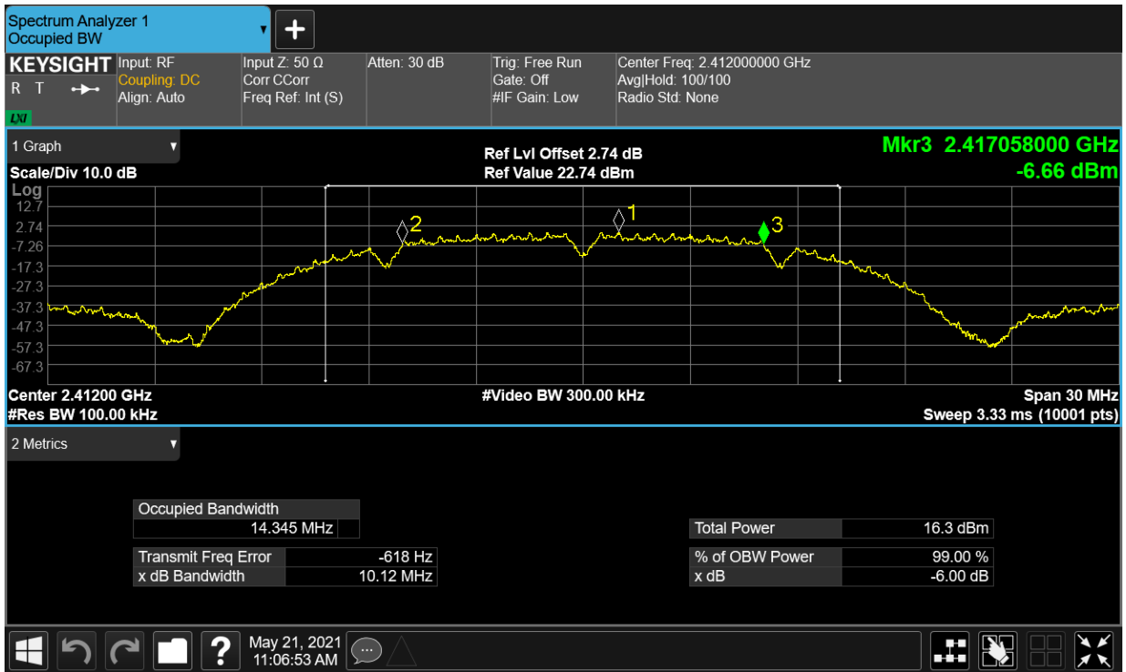
-6dB Bandwidth NVNT b 2437MHz Ant2
