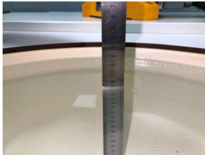
Fig. 9.2 Photo of Liquid Height for Body SAR (5000MHz~5800MHz) (depth>15cm)
