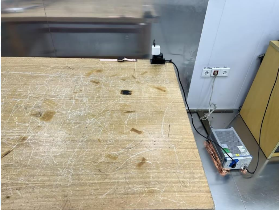
Photo of Setup for Radiated Emission (30MHz~1GHz)
