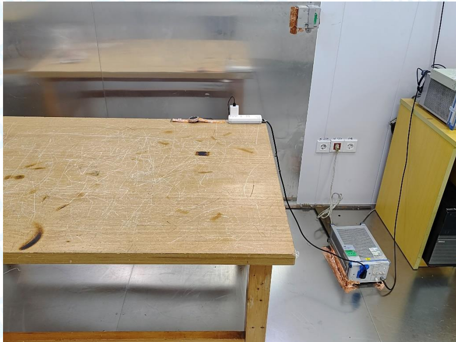
Photo of Setup for Radiated Emission (30MHz~1GHz)
