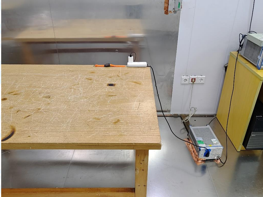
Photo of Setup for Radiated Emission (30MHz~1GHz)
