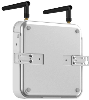
Mounting plates extended for wall mounting
