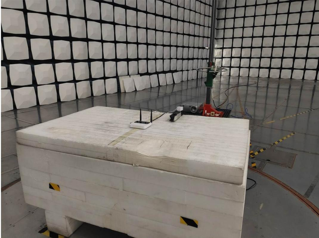
**Radiated Emission 30M-1GHz View-Powered by Adapter**
