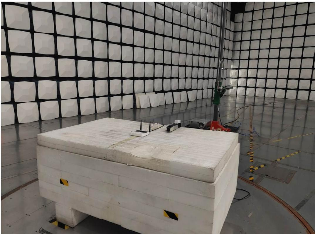
**Radiated Emission 9k-30MHz Ground-parallel View-Powered by Adapter**
