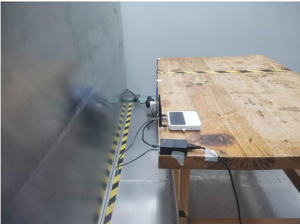
**Radiated Emission 9k-30MHz Parallel View-Powered by Adapter**
