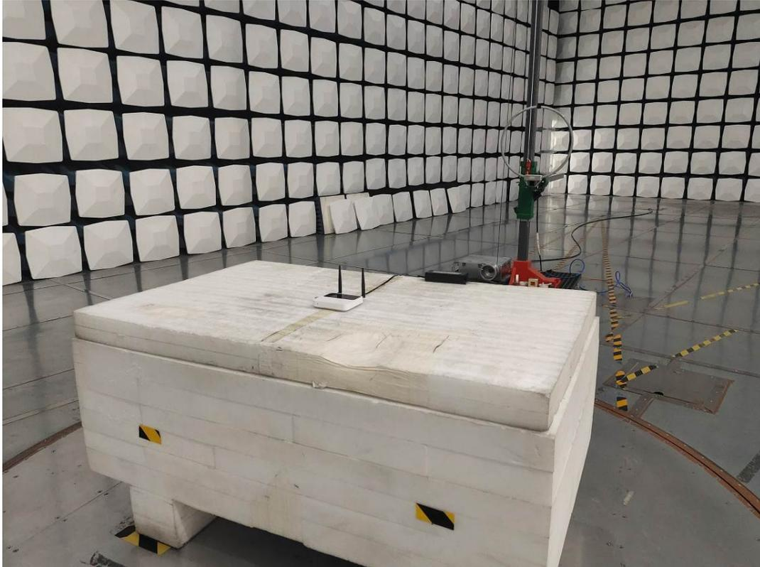
**Radiated Emission 9k-30MHz Perpendicular View-Powered by PoE**
