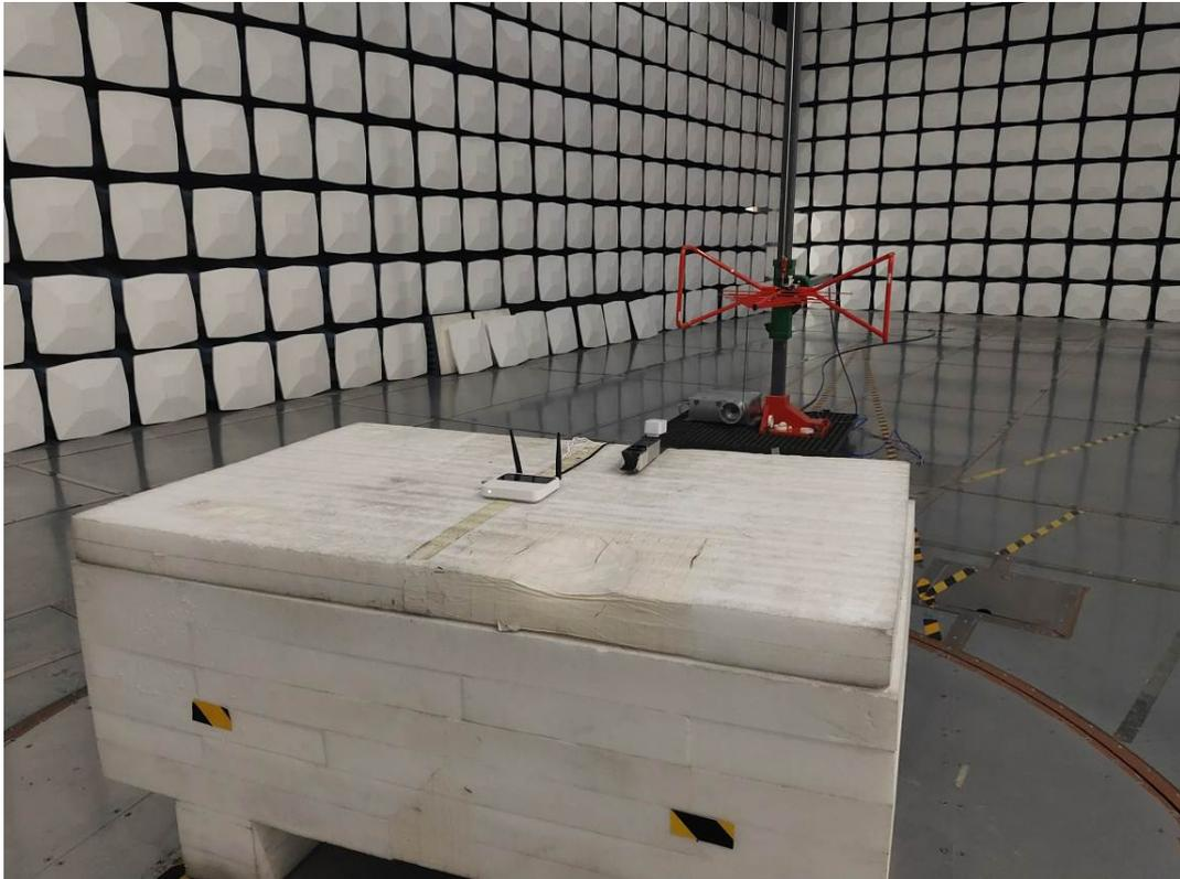
**Radiated Emission 9k-30MHz Parallel View-Powered by PoE**
