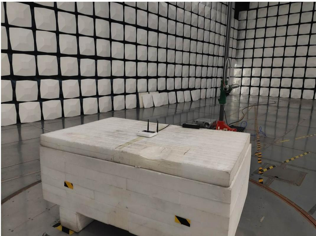
**Radiated Emission 9k-30MHz Ground-parallel View-Powered by PoE**
