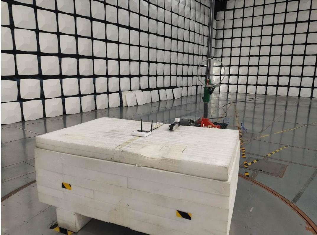
**Radiated Emission 9k-30MHz Perpendicular View-Powered by Adapter**
