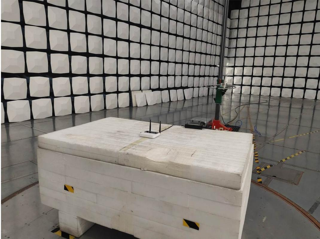
**Radiated Emission 30M-1GHz View-Powered by PoE**
