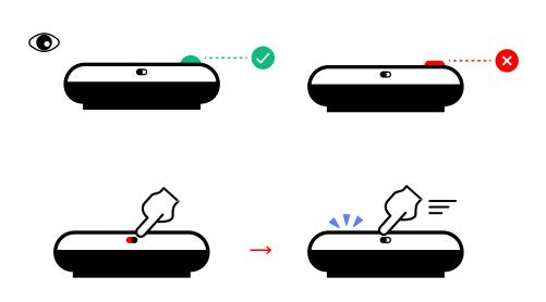
When switched on, unpaired Heatic Sensors set to the default Network ID will flash a yellow LED. If this does not occur, first ensure that the batteries are correctly installed. Next, verify that the PIR module is intact before mounting the sensor. For further assistance, contact your Butlr representative or submit a support ticket.
