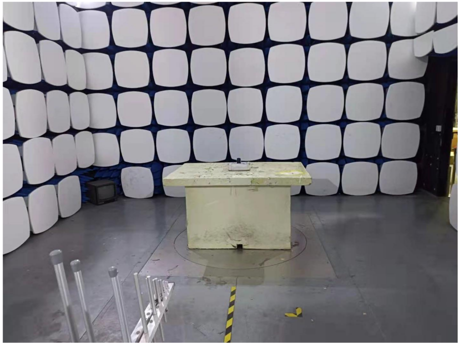
Radiation Emission Test Setup (30MHz to 1GHz)
