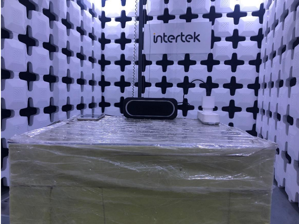
Above 1G The EUT is placed at the center of turntable
