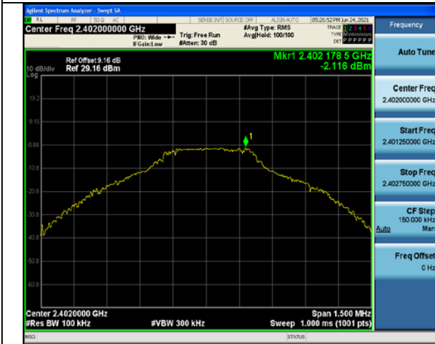
GFSK on Channel 00
