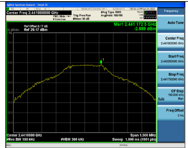
GFSK on Channel 39
