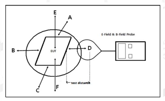
Note: Due to installation limitations no tests from the underside of the charging device (Test Position F) are required. The test position F is required when the distance is 0 cm for partable device.
