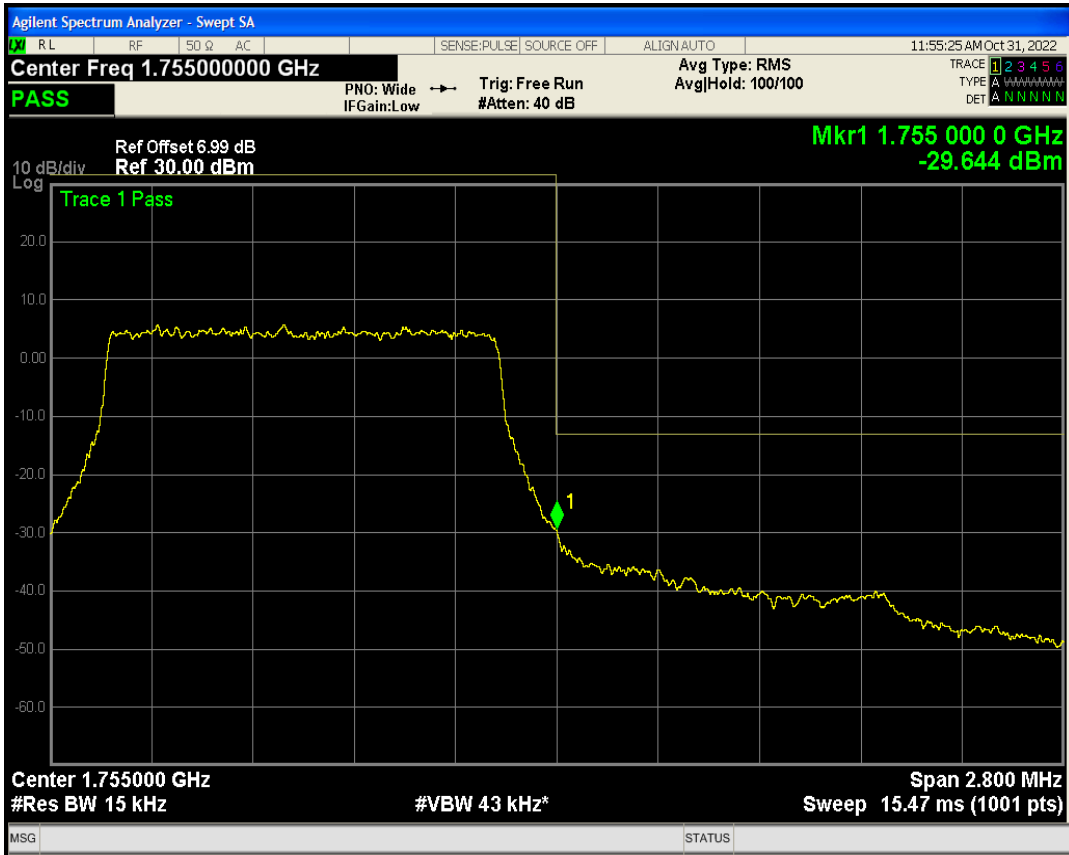
Band4 QAM16 BW=1.4MHz Channel=20393 RB Size=6 Position=#0
