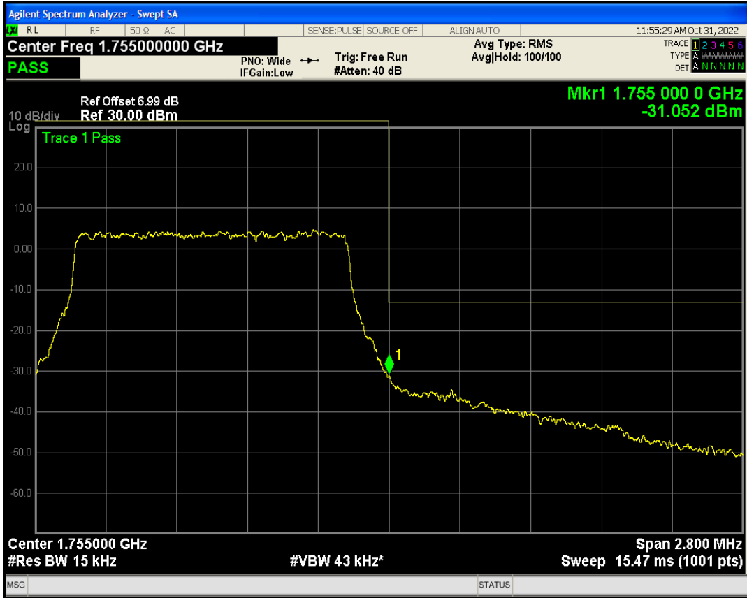
Band4 QPSK BW=3MHz Channel=19965 RB Size=15 Position=#0
