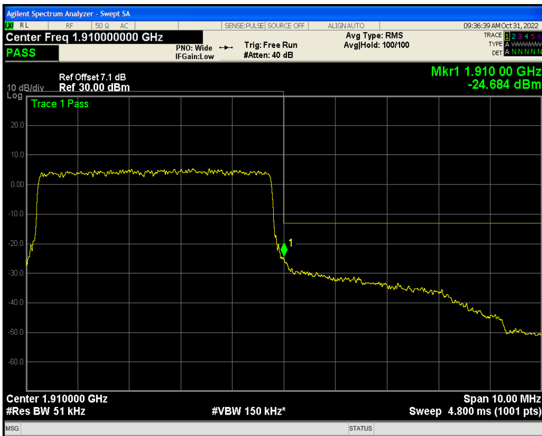
Band2 QAM16 BW=5MHz Channel=19175 RB Size=25 Position=#0
