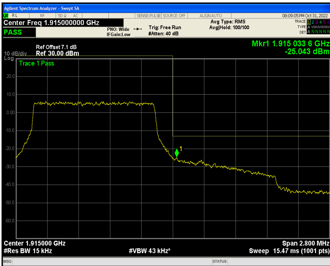
Band25 QAM16 BW=1.4MHz Channel=26683 RB Size=6 Position=#0
