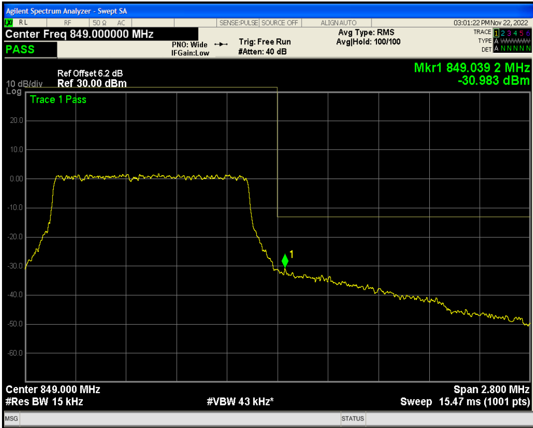
Band26(824-849) QPSK BW=3MHz Channel=26805 RB Size=15 Position=#0
