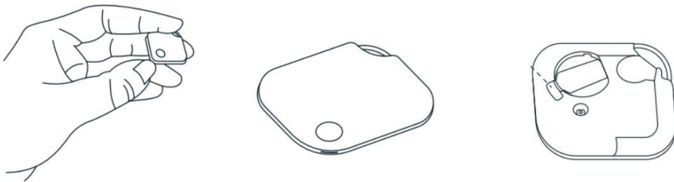
When replacing the battery, remove the shell face and replace the battery directly, with the positive electrode facing up, as shown in the figure below.
