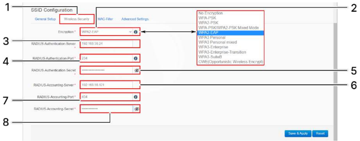
Figure 39: Basic overview of the screen to configure wireless security parameters of SSID (RADIUS)
