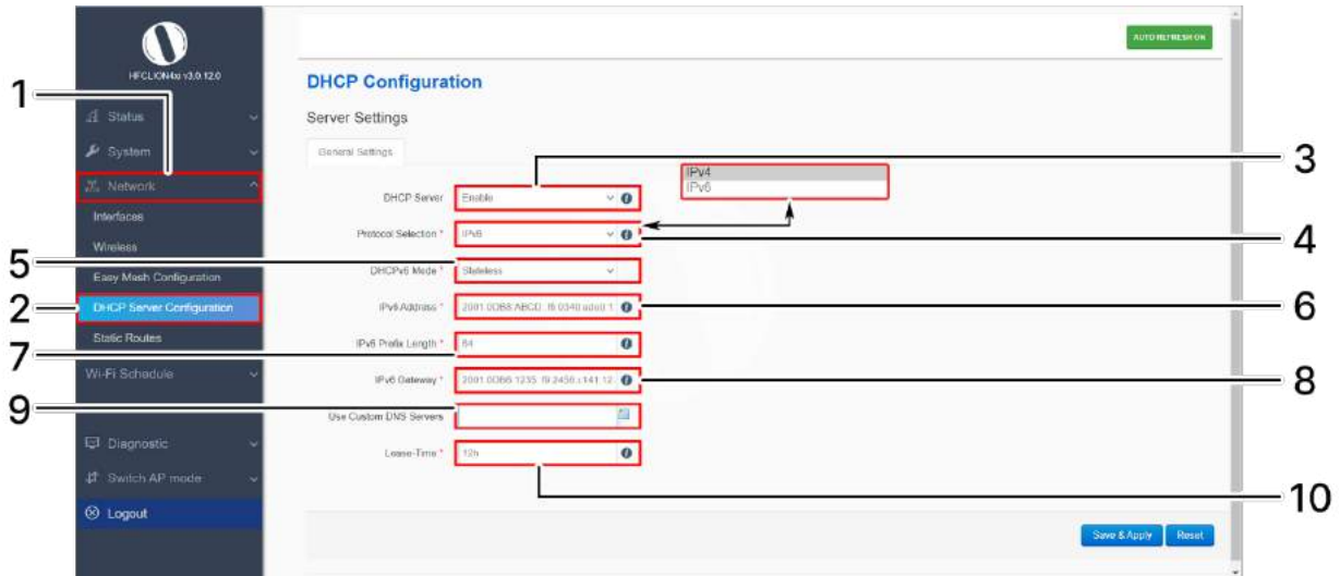
Figure 44: Basic overview of the screen to enable thick AP as DHCP server (IPv6)
