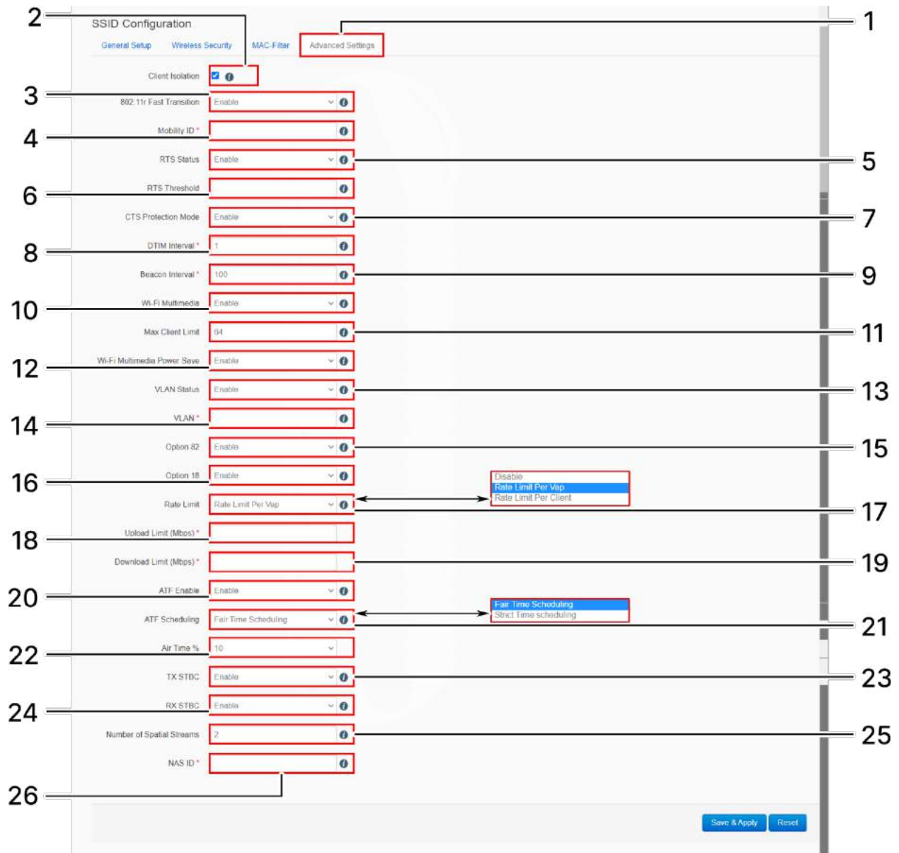
Figure 41: Basic overview of the screen to configure the advanced parameters of SSID configuration
