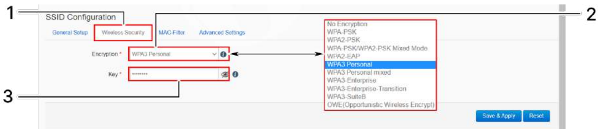
Figure 38: Basic overview of the screen to configure wireless security parameters of SSID
