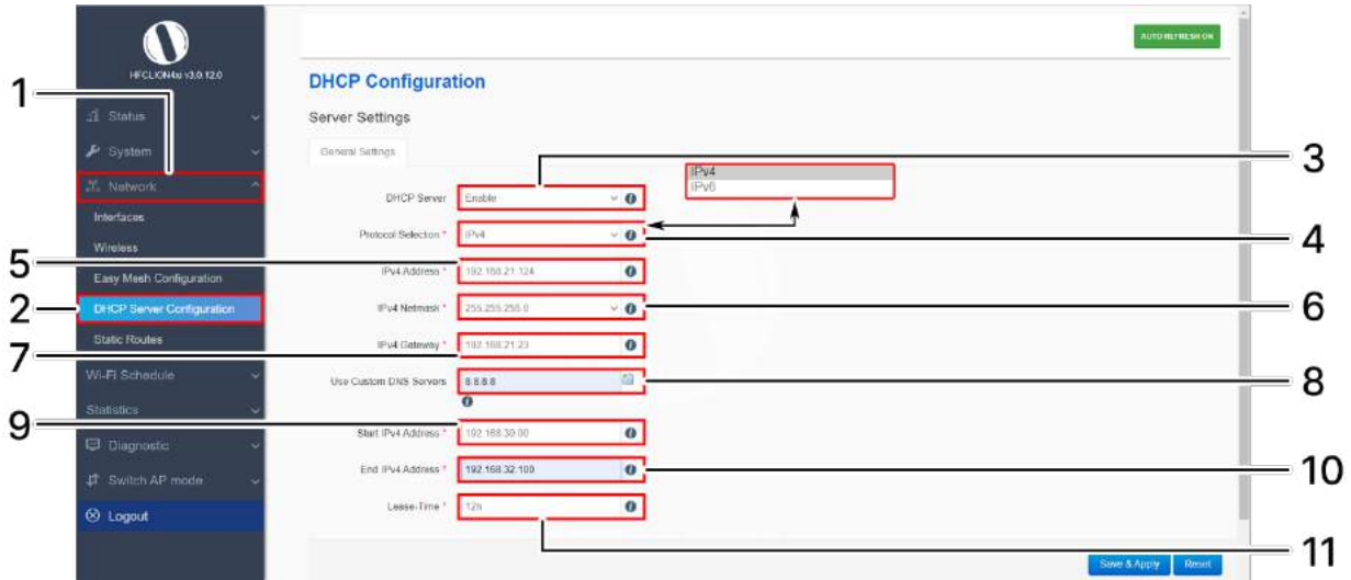
Figure 43: Basic overview of the screen to enable thick AP as DHCP server (IPv4)
