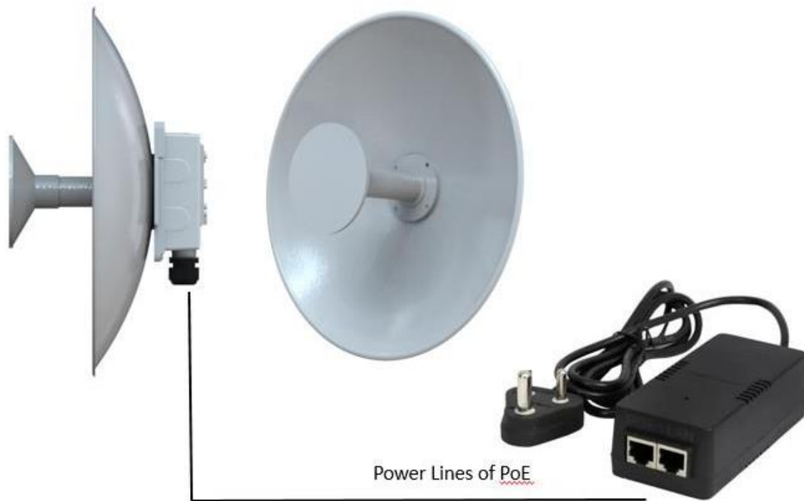
Figure 7: Basic overview of the device (UBR CPE) power up with 25dB Dish Antenna
