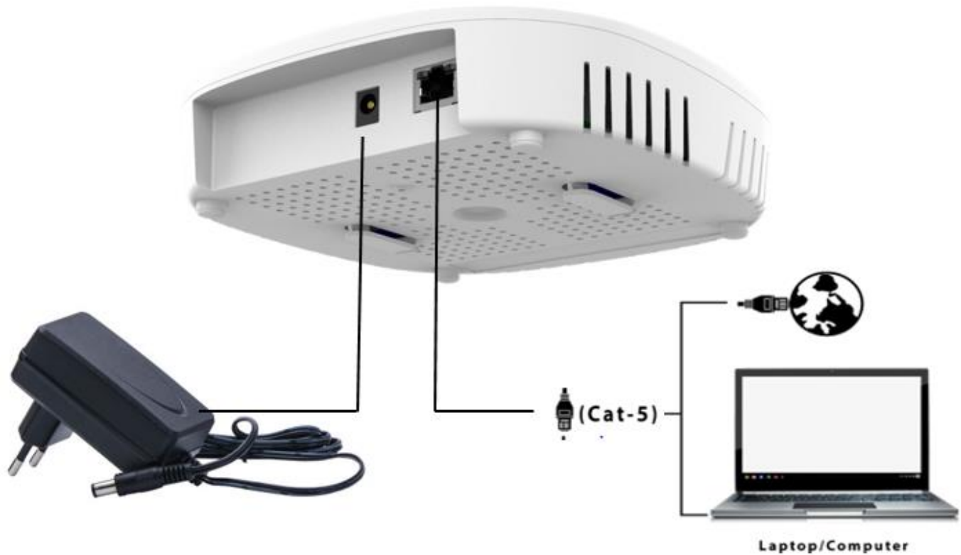
Figure 7: Connect Indoor Device to the network
