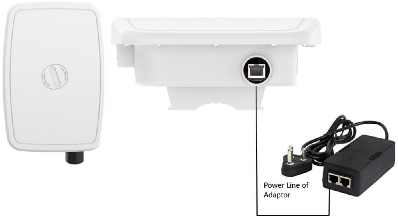
Figure 8: Power up the Outdoor device using PoE adaptor
