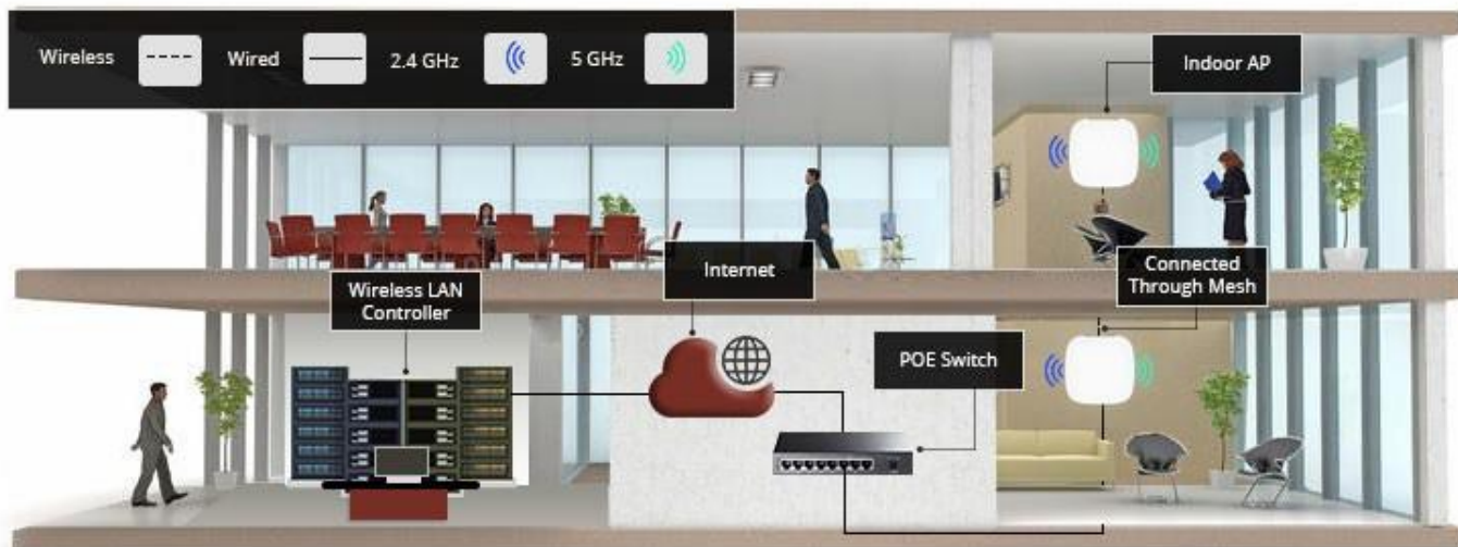
Figure 18: Use Case Diagram of Indoor AP
