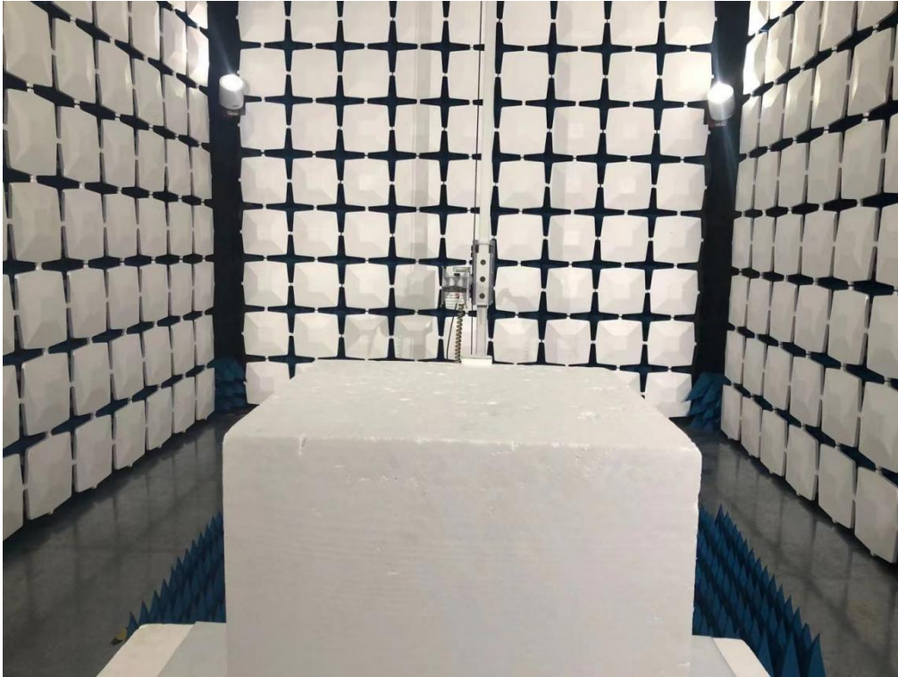
Above 1GHz for radiated emission test setup
