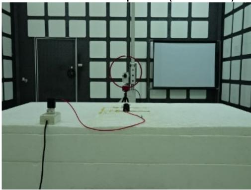
Radiated Emission Set up Photos (Below 1GHz)
