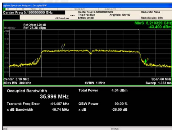
(802.11 n40) 99%Bandwidth plot on channel 46
