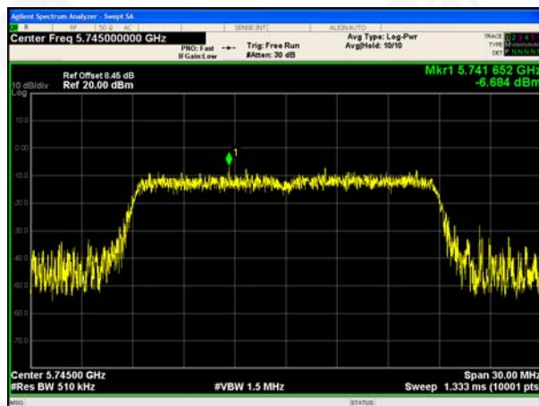
(802.11n20) PSD plot on channel 157
