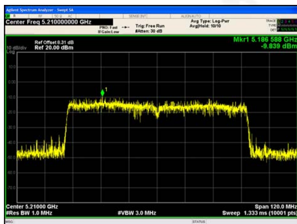
(802.11ac80) PSD plot on channel 42
