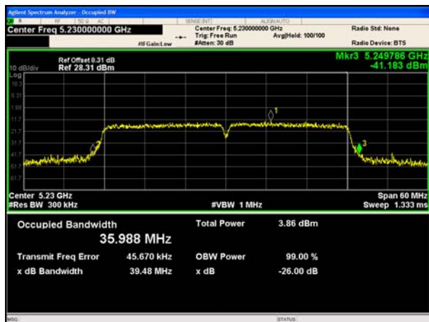
(802.11 n40) 99%Bandwidth plot on channel 46
