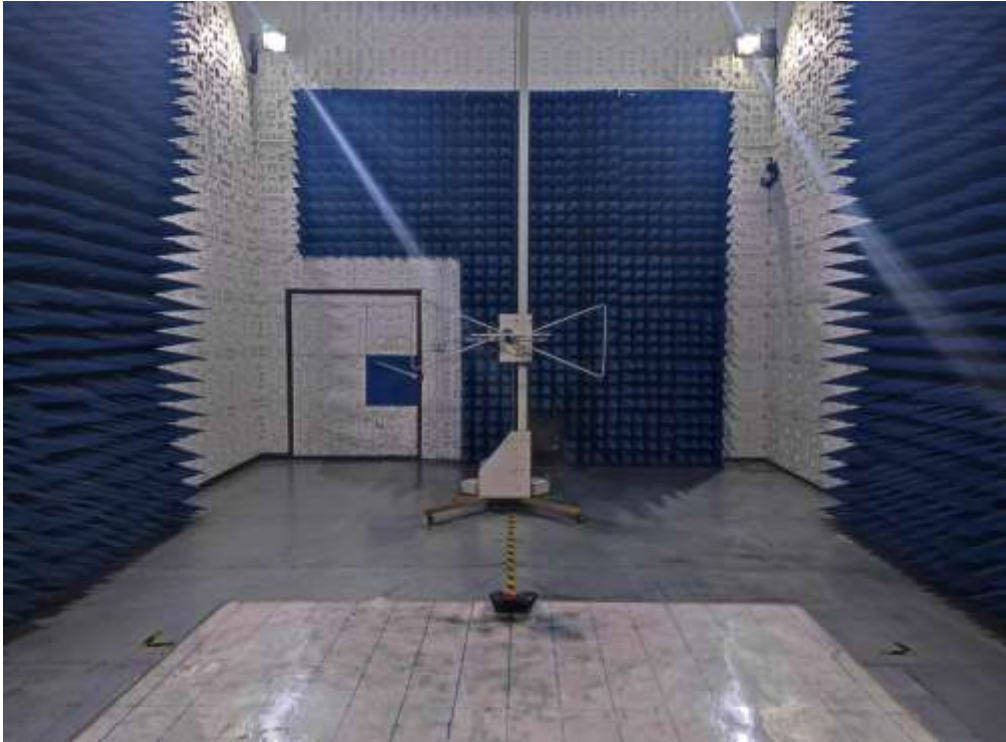
RADIATED EMISSION TEST SETUP ABOVE 1GHZ
