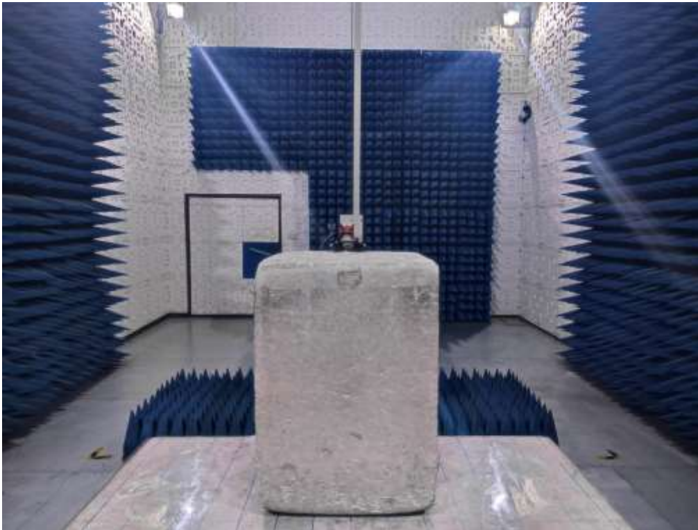
RADIATED EMISSION TEST SETUP ABOVE 1GHZ
