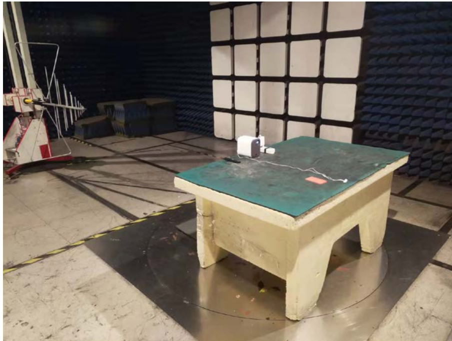
Spurious Emission Test Setup (Below 1GHz)
