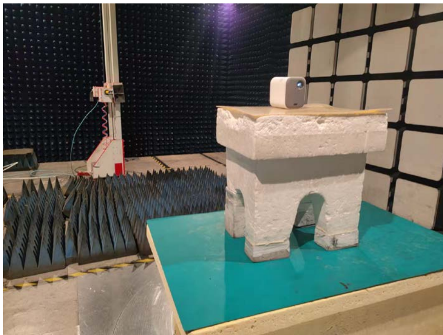
Spurious Emission Test Setup (Above 1GHz)
