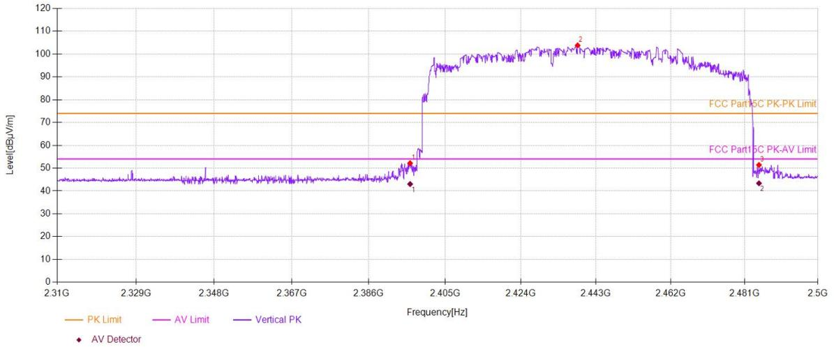
**Test Model** Spurious Emission in Restricted Band 2310-2390MHz and 2400-2483.5MHz Hopping GFSK H
