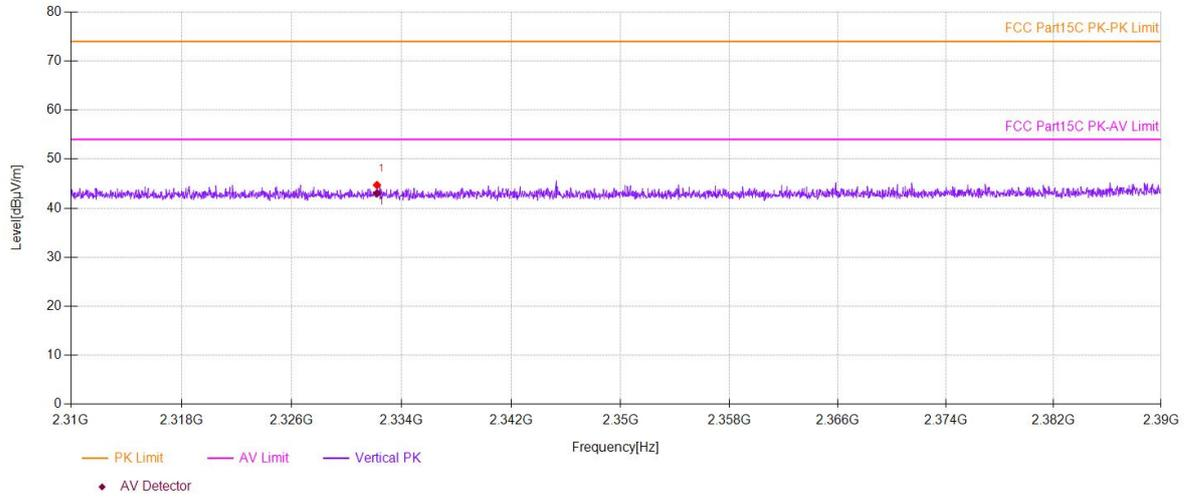
**Test Model**      **Spurious Emission in Restricted Band 2310-2390MHz**
