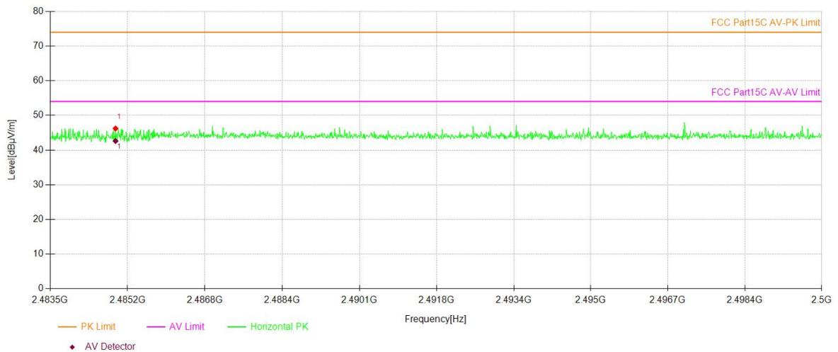
**Test Model** Spurious Emission in Restricted Band 2310-2390MHz and 2400-2483.5MHz Hopping GFSK V
