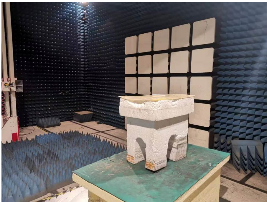
Spurious Emission Test Setup (Above 1GHz)
