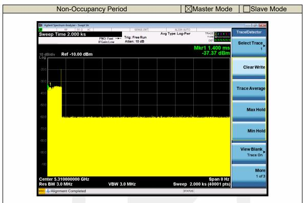
Note: During the 30 minutes observation time, UUT did not make any transmissions on a channel after a radar signal was detected on that channel by either the Channel Availability Check or the In-Service Monitoring.
