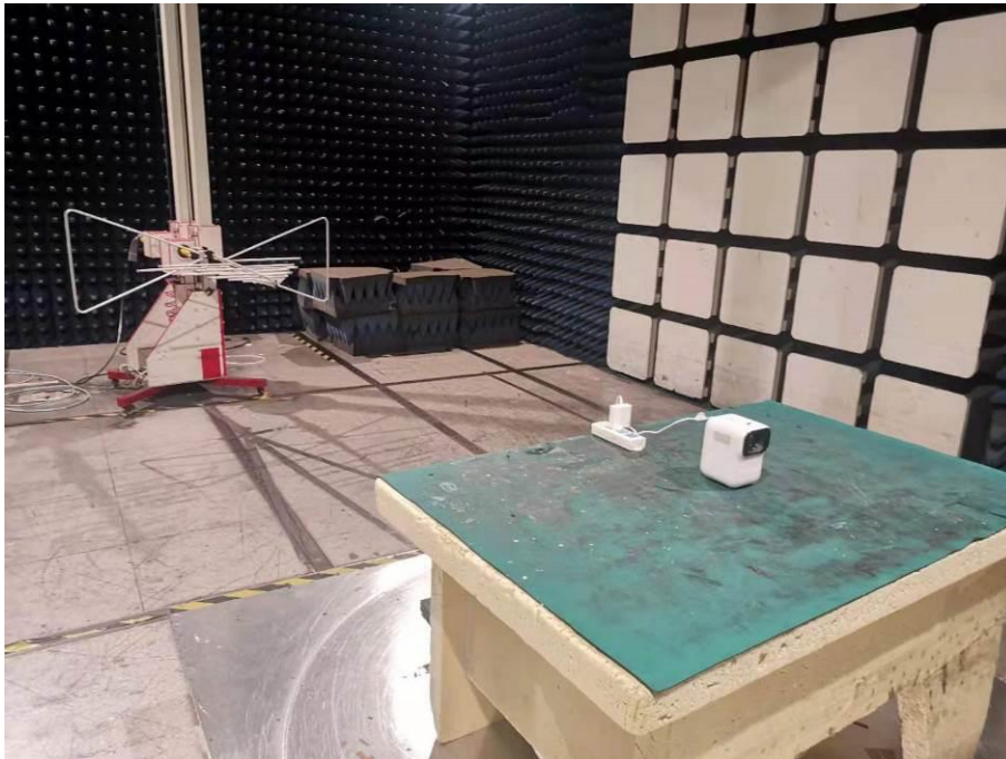
Spurious Emission Test Setup (Below 1GHz)
