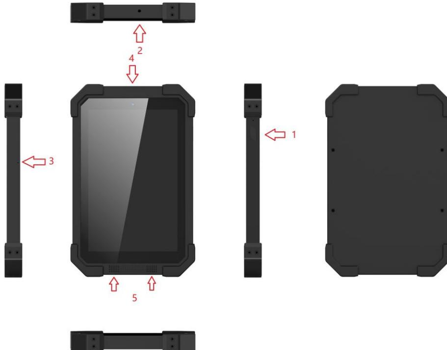
1. Power key: Press to lock or wake up the screen. Press and hold to turn the device on or off, restart it.
