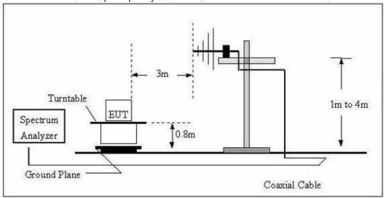
(C) Radiated Emission Test-Up Frequency Above 1GHz
