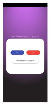
You can now verify whether your mobile is connected to the device by trying to Turn it OFF / ON. If the device could be turned OFF and turned ON, you have successfully setup your device.
