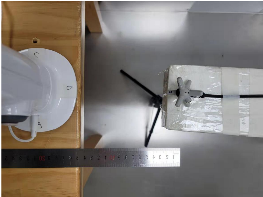
E-field Test Setup Photo of Position D(15cm)
