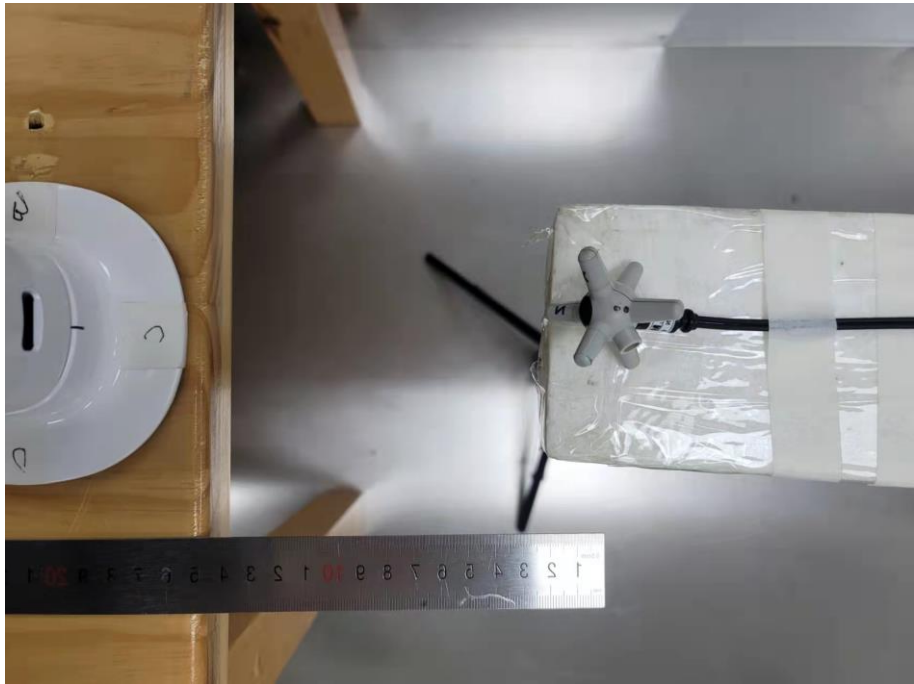
E-field Test Setup Photo of Position C(15cm)
