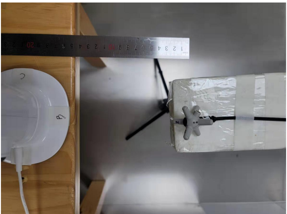
E-field Test Setup Photo of Position B(15cm)
