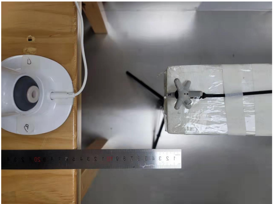
E-field Test Setup Photo of Position A(15cm)
