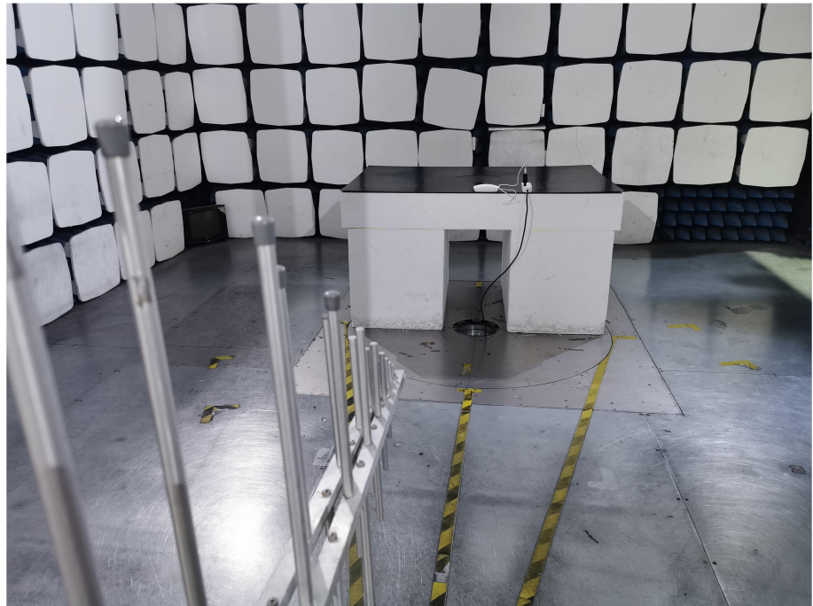
Radiation Emission Test Setup (30MHz to 1GHz)
