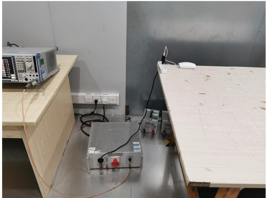
Conducted Emission Test Setup
