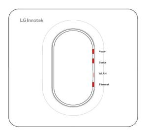
When Modules are working abnormally, three LEDs(Power, Status, Ethernet) would blink to alarm the unusual state.
