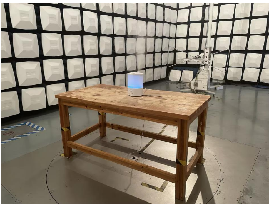
Test Setup For Radiated Emission (30MHz to 1GHz)
